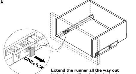
Extend the runner all the way out Unlock by pulling the black plastic peg on the runner out
