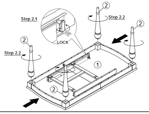
Step 3 <u>Important</u>: Ensure you have already locked the slides in Step 2 before righting the table. <u>Note</u>: When moving the table, remove leaf, close table top and lock the slides, then move by gripping or lifting the legs or underframe.
