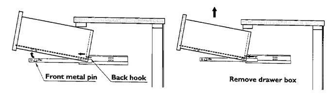
Hold both runners with both of your hands. Carefully lift the drawer front up from the front metal pin, then slide forward to remove from back hooks
